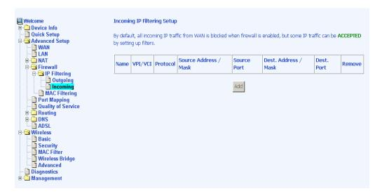
Enter a filter name, information about the source address (from the WAN side), and information about the destination address (to the LAN side). Select the protocol and WAN interface, and then click on **Save/Apply** to add the setting.
